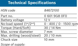
2 x 12V 1.5 Ah Li-ion Batteries, 1 Charger, Carry Case, Accessory set, 6 metal drill bit, 4 wood drill bit, 10 screw driver bit and 1 screw driver bit holder
