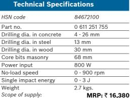
Scope of supply: Auxillary Handle; Depth Gauge;
